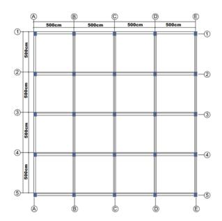
Figure 11. The blueprint of the sample RC building.
