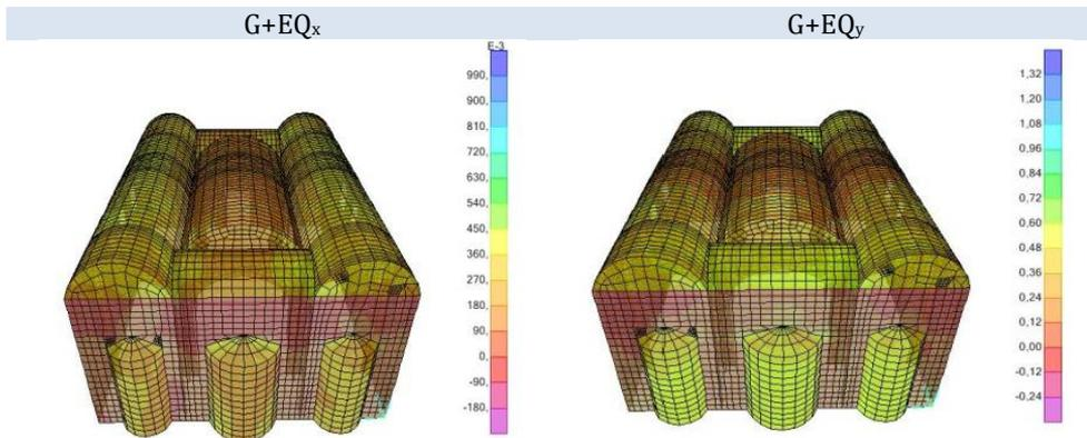
Figure 16.  $S_{12}$  tensile stresses distribution, (MPa)
