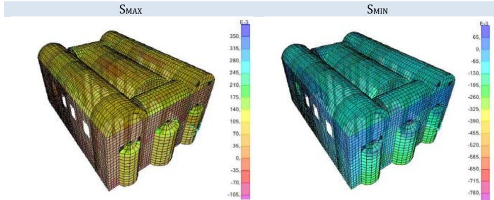
Figure 11.  $S_{MAX}$  and  $S_{MIN}$  Stresses diagram, (MPa)
